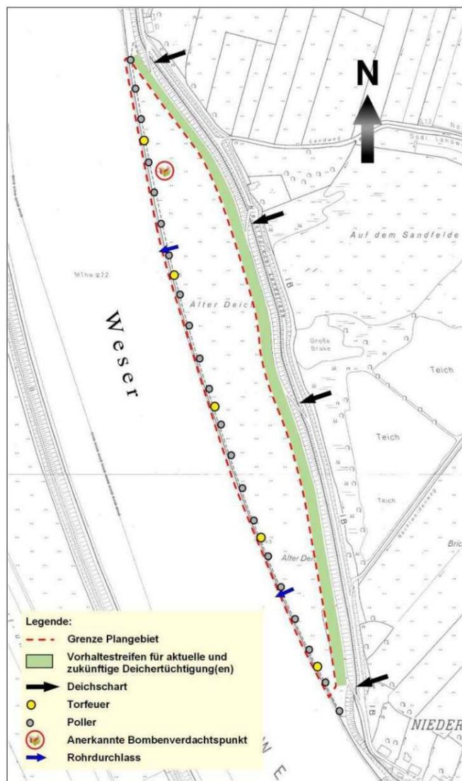
The limits of the planning area are defined by the land required for the expected dike repair as well as the mean low tide (MTnw). This means that the area's border to the east runs parallel to the present foot of the Weser dike at a distance of 25 m from this. In the west the border runs along the MTnw line (-1.57 m MSL).
